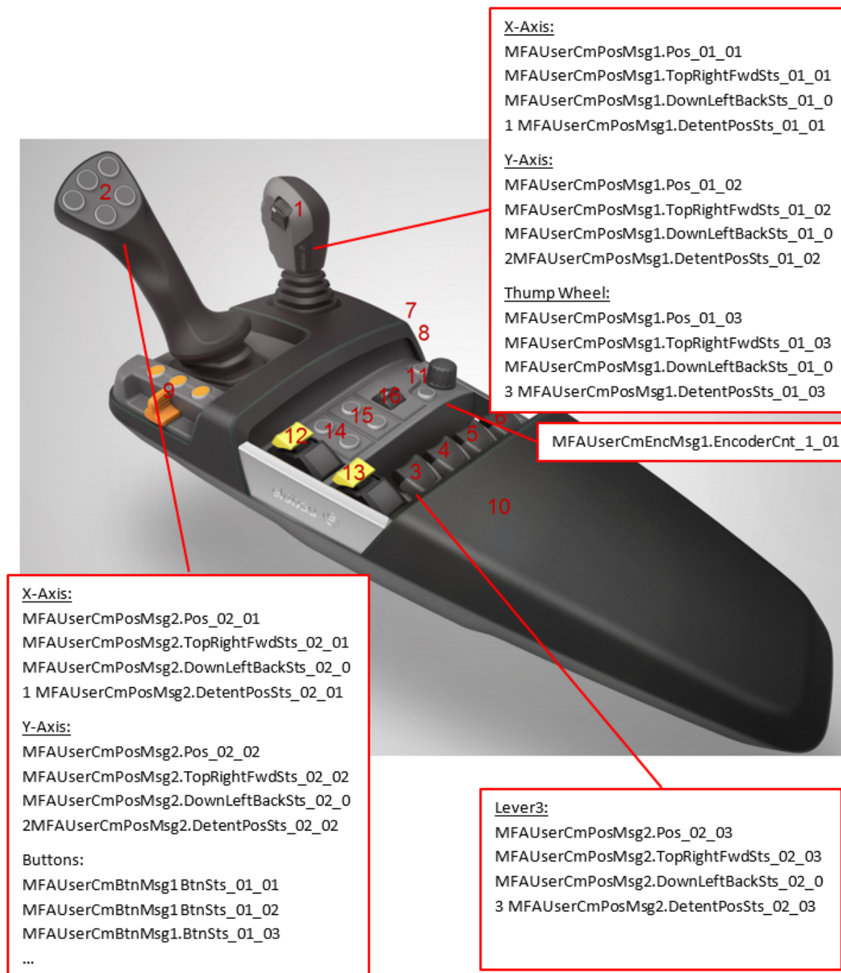
Figure 4 CAN mapping example
